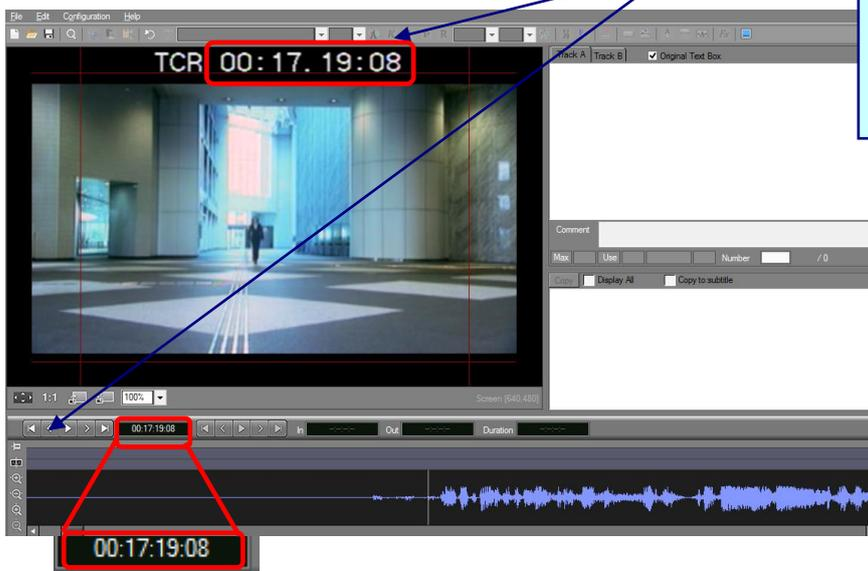
7. Make sure the time codes of the image and SST G1 Pro are synchronized.
